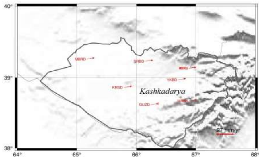
Figure 3. Horizontal velocities of GNSS stations relative to ITRF 2014
