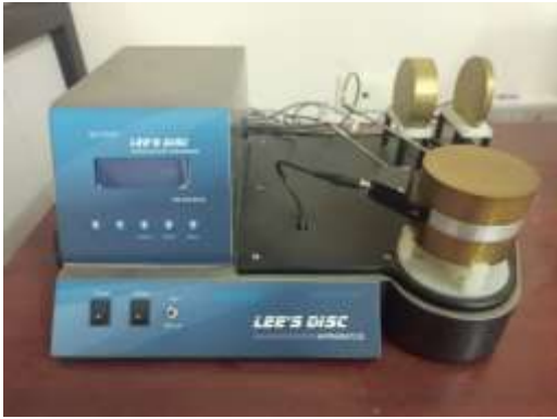
Fig 6 Lee Disc Apparatus
