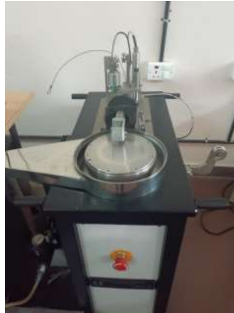
Fig 7 Pin On Disc Apparatus
